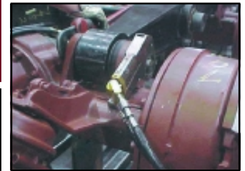
Patented multi-axis swivel, provides for better accessibility and prevents hose kinking.
